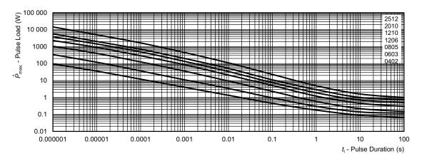
Maximum pulse load, single pulse; applicable if  $\bar{P} \to 0$  and  $n \le 1000$  and  $\hat{U} \le \hat{U}_{max}$ ; for permissible resistance change equivalent to 8000 h operation
