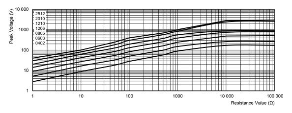
Pulse load rating in accordance to EN 60115-1, 4.27; 10 µs / 700 µs; 10 pulses at 1 min intervals; for permissible resistance change 1 %
