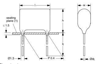
Dimensions in mm (1) Hole  $\varnothing$  1.0 for d<sub>t</sub> = 0.6 mm
