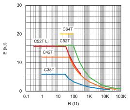
Repetitive Operation Energy as a Function of  $R_n$ Pulse Duration < 100 ms E = f(R)
