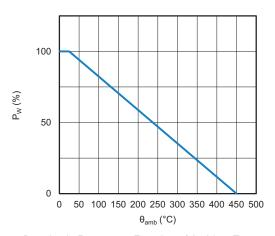
Derating in Power as a Function of Ambient Temperature
