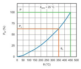
$\label{eq:PW} \begin{array}{l} \text{Power P}_W \text{ as a Function of Surface Temperature} \\ P(W) = f \text{ (Temperature Surface)} \end{array}$
