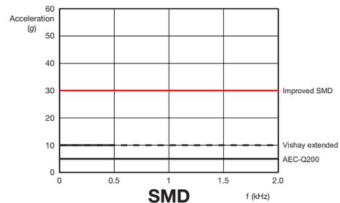
During vibrations, the heavy parts could easily break loose from the PCB. Therefore, care has to be taken in regards to PCB thickness and fixation of the capacitor to the board. Relatively unknown is the appearance of resonances during vibrations. Cases have been reported in which the actual measured vibrational accelerations at the capacitor location gained up to a factor of 50 relative to the pre-set test conditions.
