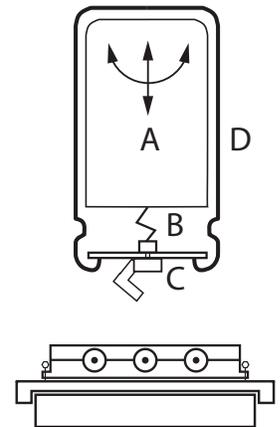
Improvements to the internal robustness of the capacitor can be made by providing a more rigid axial or radial fix for the winding element. Some Vishay series improve the vibration sensitivity capability up to 50 g, which is five times the requirement of the IEC test.
