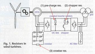
are a perfect choice. The pulse energy for the pre-charge resistor is typically about 5 J for capacitance of 10 µF and dc voltage of 690 V.
