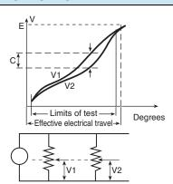
It is the maximum deviation between the actual voltage outputs of 2 or more pot modules in the same assembly. It is expressed as a percentage of the total applied voltage, or in dB attenuation.
