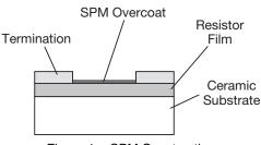
Figure 1. - SPM Construction
