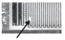
Figure 2. - Electrolytic corrosion caused by reaction of moisture combined with low power on Nichrome resistive element.
