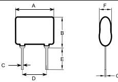
On front side: Vishay logo and ohmic value (in  $\Omega$ ). On back side: manufacturing code and tolerance (in %)
