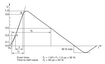
Fig. 3 - Waveform of Open-circuit Voltage (1.2/50 µs) at the Output of the Generator with no CDN connected (waveform definition according to IEC 60060-1)
