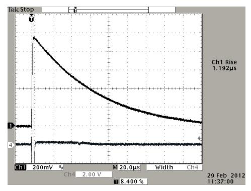
Fig. 2 - 1.2/50 µs Waveform Verification
