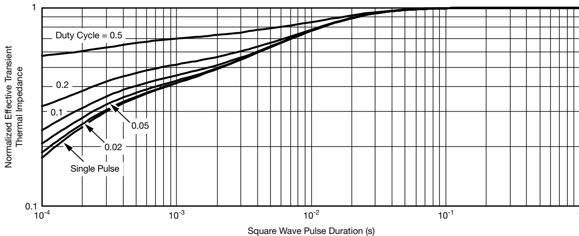
Normalized Thermal Transient Impedance, Junction-to-Case
