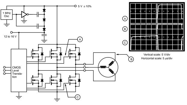
Figure 1. 5-Volt, 3-Phase Motor Drive
