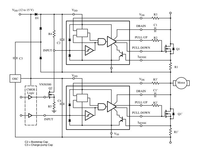
Figure 4. Si9910DY Adaptive MOSFET Gate Driver
