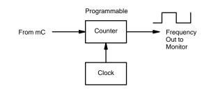
FIGURE 4. Saturated Oxygen Simulation Circuit
