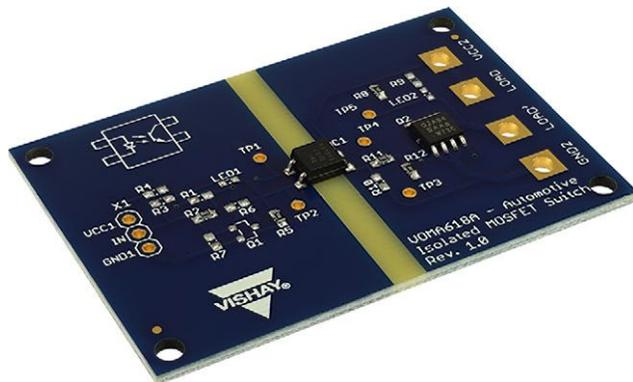
Fig. 1 - VOMA618A - Automotive Isolated MOSFET Switch Evaluation Board Picture
