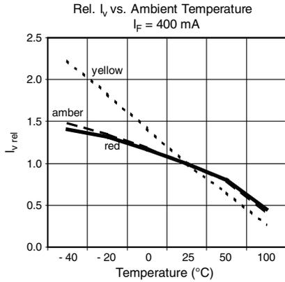
Fig. 8 - Relative Luminous Intensity vs. Ambient Temperature
