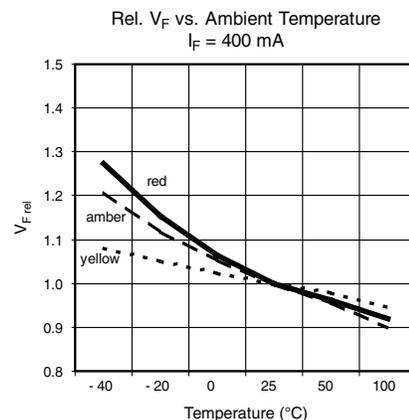
Fig. 6 -  $V_f$  over Temperature for AllInGaP Based Devices
