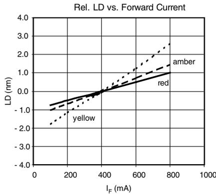
Fig. 13 - Dominant Wavelength vs. Forward Current
