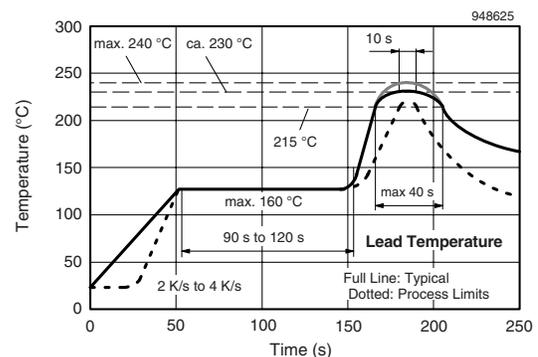
Fig. 21 - Recommended Lead (Pb)-free IR-reflow Profile for Lead (Pb)-free Soldering
