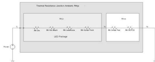
Fig. 18 - The Thermal Resistance  $R_{thja}$  as a Summary of Individual Parts
