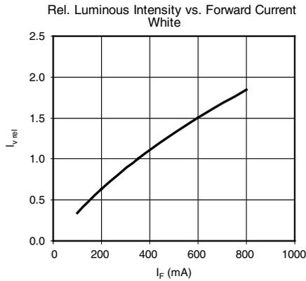
Fig. 14 - White: Luminous Intensity vs. Forward Current
