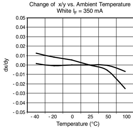
Fig. 11 - Color Coordinates x, y vs. Ambient Temperature
