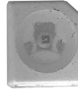
Fig. 5 - Acceptable Foreign Particle Level on a Silicone Casted LED
