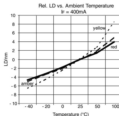
Fig. 7 - Dominant Wavelength vs. Ambient Temperature
