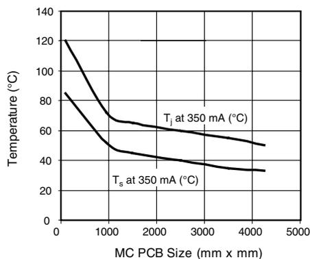
Fig. 19 - The Effect of Heat Sink Size on Junction and Solder Point Temperature
