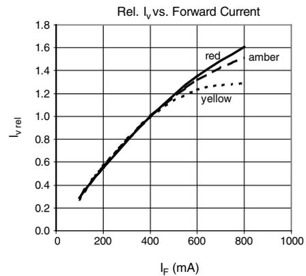
Fig. 12 - LOP vs. Forward Current
