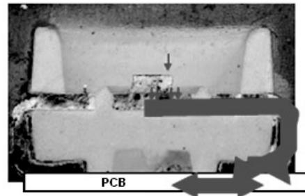
Fig. 17 - The Way the Heat Goes out of the LED via Leadframe to the PCB
