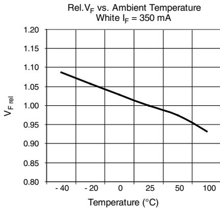
Fig. 9 -  $V_F$  vs. Ambient Temperature for White
