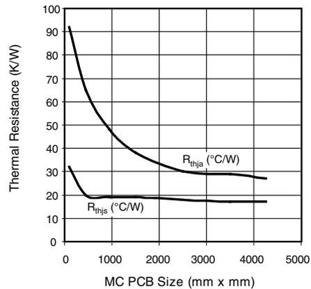
Fig. 20 - Effect of Heat sink size on  $R_{thjs}$  and  $R_{thja}$
