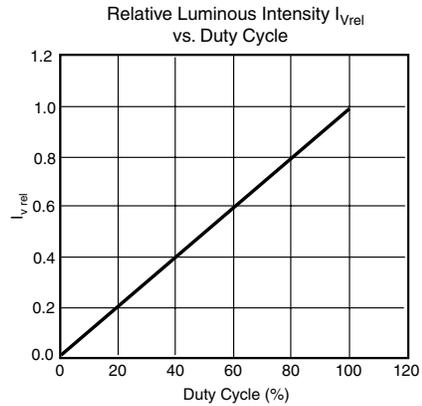
Fig. 16 - Relative Luminous Intensity vs. Duty Cycle
