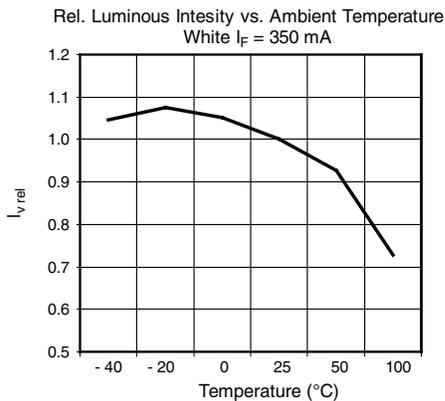
Fig. 10 - Relative Luminous Intensity vs. Ambient Temperature for White
