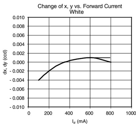
Fig. 15 - White: X, Y vs. Forward Current
