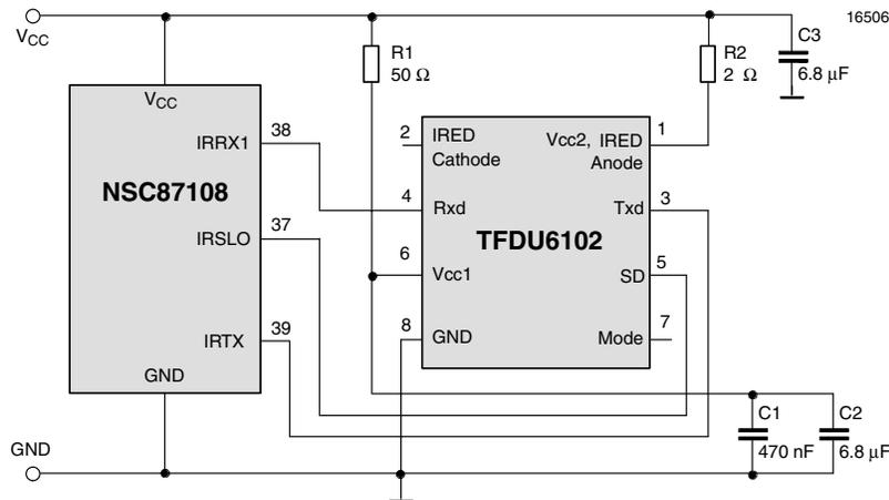
Figure 2. Application Example using NSC87108
