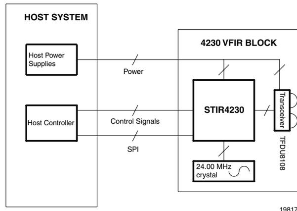
Figure 5. Block diagram of the USB to IrDA interface
