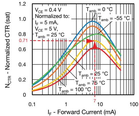
Fig. 7 - Normalized Current Transfer Ratio (saturated) vs. Forward Current
