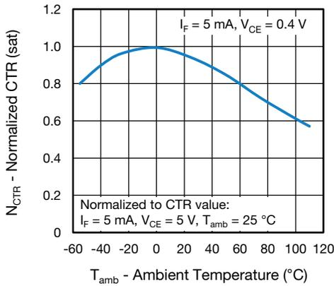
Fig. 2 - Normalized Current Transfer Ratio (saturated) vs. Ambient Temperature
