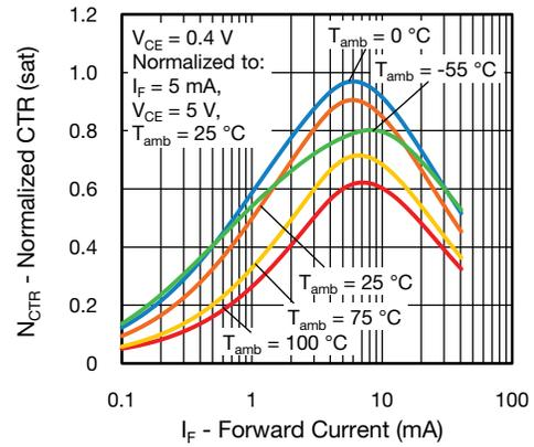
Fig. 4 - Normalized Current Transfer Ratio (saturated) vs. Forward Current
