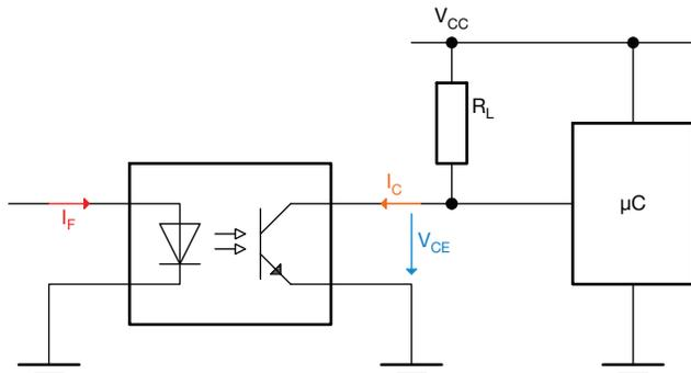
Fig. 6 - VOL617A-3 to Microcontroller Interface
