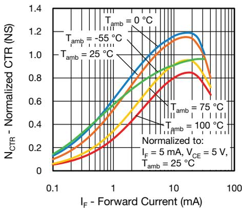
Fig. 3 - Normalized Current Transfer Ratio (non-saturated) vs. Forward Current
