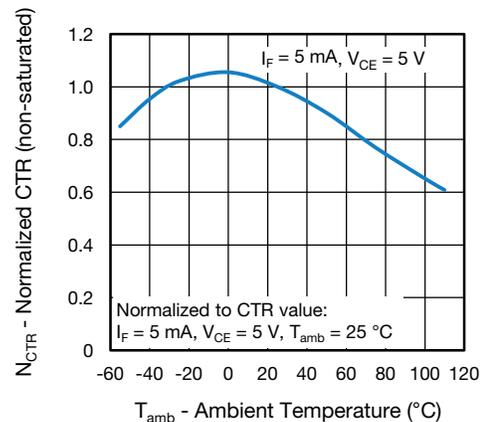
Fig. 1 - Normalized Current Transfer Ratio (non-saturated) vs. Ambient Temperature
