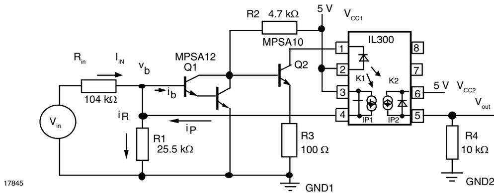
Fig. 2 - Discrete Isolation Amplifier
