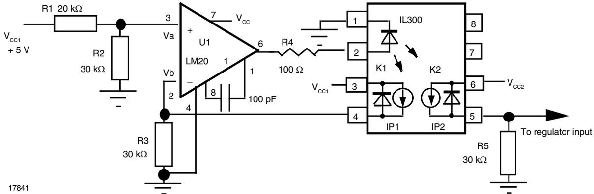
Fig. 10 - + 5 V Isolated Feedback Amplifier
