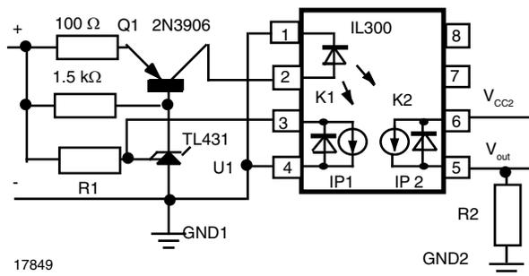
Fig. 16 - Shunt Voltage Regulator Isolation Amplifier
