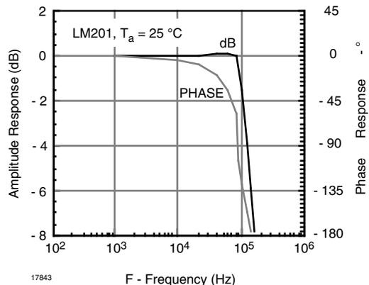
Fig. 12 - LM201 Phase and Frequency Response
