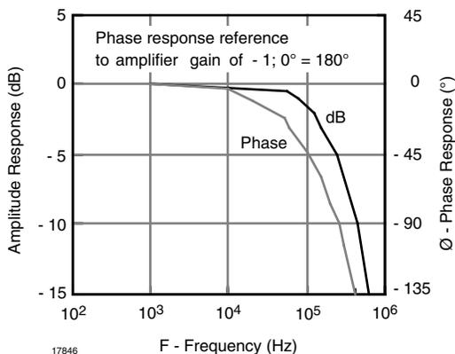
Fig. 13 - Discrete Isolation Phase and Frequency Response
