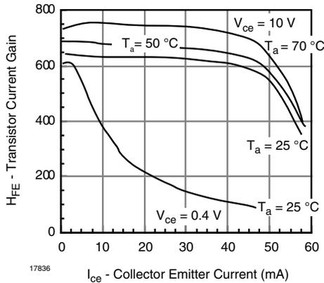
Fig. 5 - Phototransistor H
