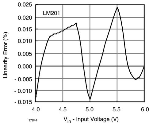
Fig. 1 - LM201 Linearity Error
