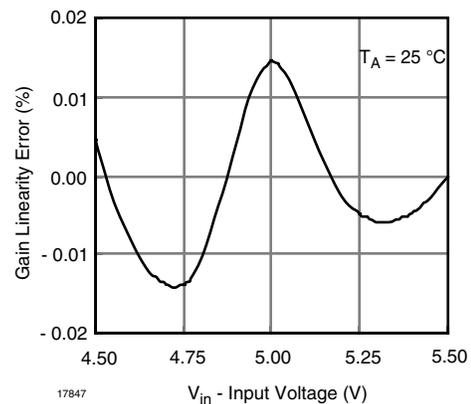
Fig. 14 - Discrete Isolation Linearity Error
