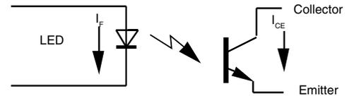
A. Simple Phototransistor
