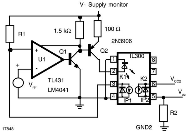
Fig. 15 - Shunt Voltage Regulator
