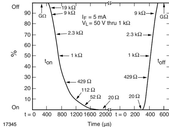
Fig. 1 - Dynamic Switching Resistance
