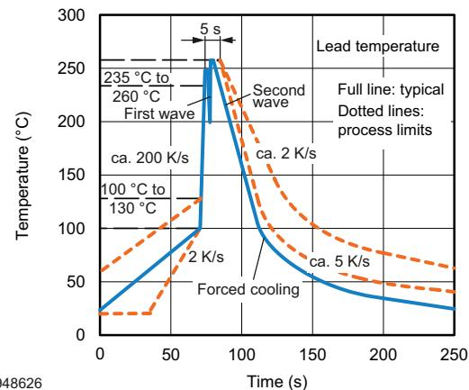
Fig. 20 - Wave Soldering Double Wave Profile
