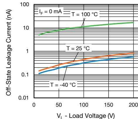
Fig. 11 - Off-State Leakage Current vs. Load Voltage
