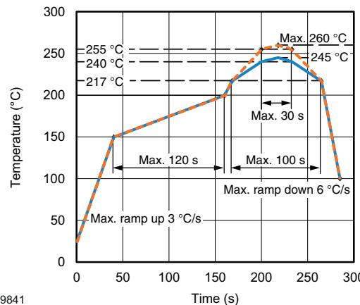
Fig. 21 - Lead (Pb)-free Reflow Solder Profile
