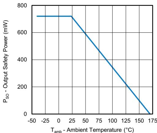
Fig. 3 - Output Safety Power vs. Ambient Temperature
