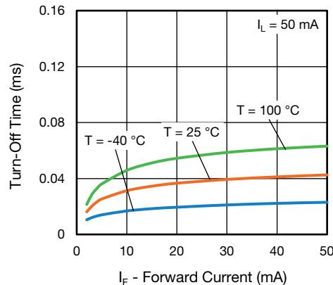
Fig. 14 - Turn-Off Time vs. Forward Current
