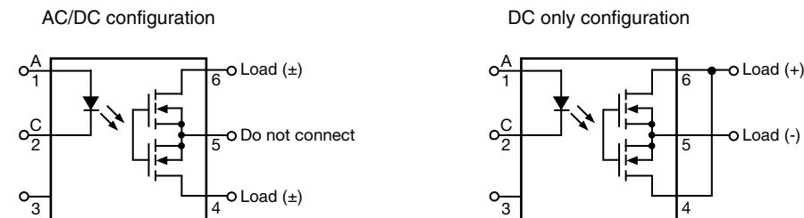
Fig. 1 - Pin Configuration
