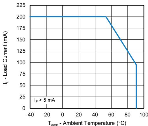
Fig. 5 - Load Current vs. Ambient Temperature
