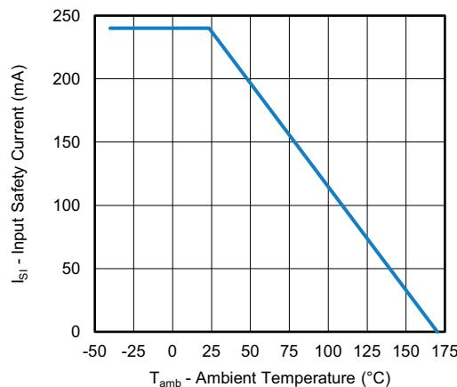
Fig. 4 - Input Safety Current vs. Ambient Temperature
