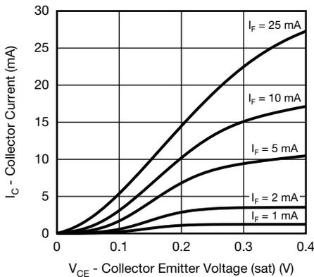
Fig. 3 - Collector Current vs. Collector Emitter Voltage (saturated)
