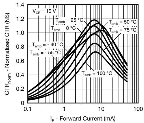
Fig. 4 - Normalized CTR vs. Forward Current (non-saturated)
