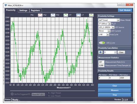
Fig. 29 - HRM Pulses Measured With the VCNL3036 Sensor Board
