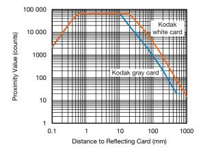
Fig. 12 - Proximity Value vs. Distance for 8T and 200 mA
