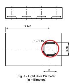
The diameter needs to be increased with the distance between the sensor and cover glass according to the following calculation:
