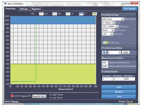
2. If a finger is placed directly on the small plastic cover, the 300 offset counts increase to more than 1000 counts
