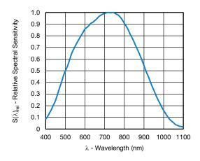
Fig. 9 - Normalized Spectral Response
