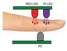
Fig. 32 - Sensing in Transmissive Mode
