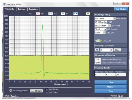
4. Just one or two measurements above the threshold will not activate the interrupt
