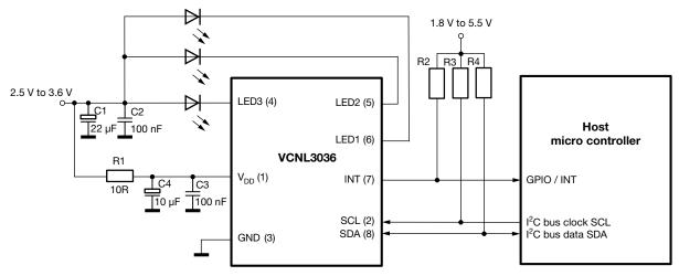
Fig. 4 - Circuitry With Just One Common Power Supply Source
