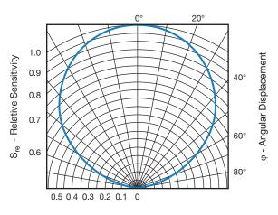
Fig. 5 - Angle of Half Sensitivity of the Photodiode
