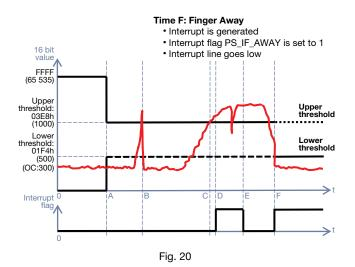
Time E: µC Awake, Threshold Reset Interrupt is cleared Interrupt flag prox\_th\_top programmed to 1 • Lower interrupt threshold = 500 Interrupt flag prox\_th\_bottom programmed to 1 16 bit value • High limit and low limit flags = 0 FFFF (65 535) Upper threshold: 03E8h (1000) Upper threshold Lower threshold: 01F4h (500) Lower threshold (OC:300)  $\geq$ С Interrupt 0 flag 🔨 0
