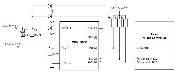
Fig. 3 - Circuitry With Two Separate Power Supply Sources
