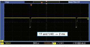
Fig. 13 - Proximity Measurements With PS\_Duty = 1/40
