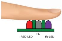
Fig. 33 - Sensing in Reflective Mode
