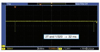
Fig. 14 - Proximity Measurements With PS\_Duty = 1/320
