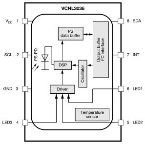
Fig. 2 - VCNL3036 Detailed Block Diagram
