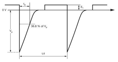
Fig. 4 - JASO D001-94 Type B and E
