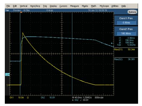
Fig. 10 - With the Applied Condition of 101 V U<sub>s</sub>, 12 V U<sub>B</sub>, and 1.25  $\Omega$  Line Impedance, as Specified by ISO-16750-2 test A, the Peak Current is 51.3 A and the Actual Clamped Current is 50.3 A.
