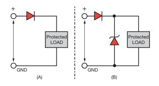
Fig. 1 - Basic Polarity Protection Circuits
