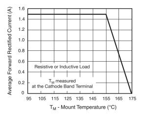
Fig. 5 - The Maximum Forward Current Derating Curve of an AS1P on a 5 mm x 5 mm Cu Pad with a FR-4 PCB
