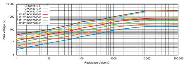
Pulse load rating in accordance to EN 60115-1, 4.27; 10  $\mu$ s / 700  $\mu$ s; 10 pulses at 1 min intervals; for permissible resistance change 1 %
