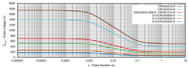
Maximum pulse voltage, single and continuous pulses; applicable if  $\hat{P} = \hat{P}_{\text{max}}$ ; for permissible resistance change equivalent to 8000 h operation
