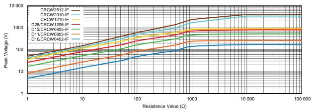
Pulse load rating in accordance to EN 60115-1, 4.27; 1.2  $\mu$ s / 50  $\mu$ s; 5 pulses at 12 s intervals; for permissible resistance change 1 %
