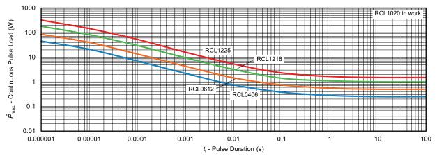
Maximum pulse load, continuous pulses; applicable if  $\overline{P} \leq P(v_{amb})$  and  $\hat{U} \leq \hat{U}_{max}$ ; for permissible resistance change equivalent to 8000 h operation
