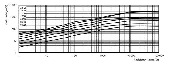
Pulse load rating in accordance to EN 60115-1, 4.27;  $10 \mu s / 700 \mu s$ ; 10 pulses at 1 min intervals; for permissible resistance change 1 %
