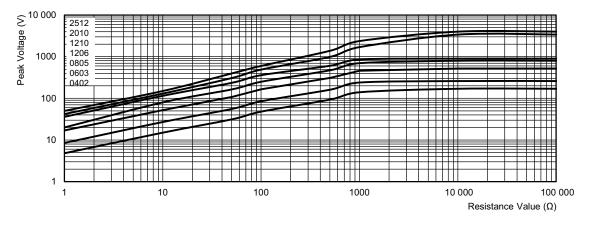
Pulse load rating in accordance to EN 60115-1, 4.27; 1.2  $\mu s$  / 50  $\mu s;$  5 pulses at 12 s intervals; for permissible resistance change 1 %
