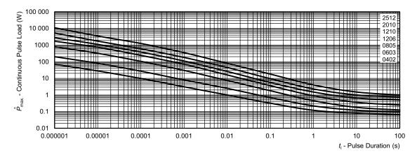
Maximum pulse load, continuous pulses; applicable if  $P \le P(\vartheta_{amb})$  and  $\hat{U} \le \hat{U}_{max.}$ ; for permissible resistance change equivalent to 8000 h operation
