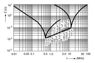
Impedance (Z) as a function of frequency (f) at  $T_a$  = 20 °C (average). Measurement with lead length 6 mm.
