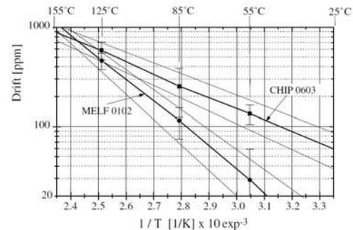
Fig. 6 - Arrhenius plots of thin film SMD resistors after 1000 h endurance tests
