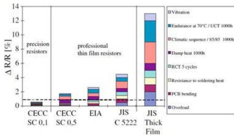
Fig. 3 - Comparison of international specifications of film resistors.
