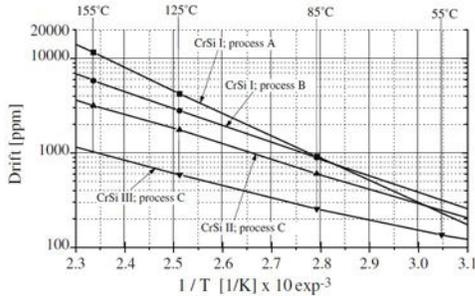
Fig. 10 - Comparison of Arrhenius plots (1000 h) from different CrSi thin film systems and different manufacturing processes
