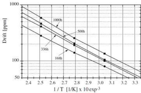
Fig. 7 - Time-dependencies of Arrhenius plots for CHIP 0603 (CrSi thin film)
