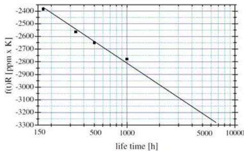
Fig. 8 - Time-dependence of  $f(t)R$  for CrSi thin film CHIP resistors size 0603
