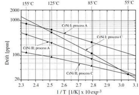
Fig. 11 - Comparison of Arrhenius plots (1000 h) from different CrNi thin film systems and different manufacturing processes.
