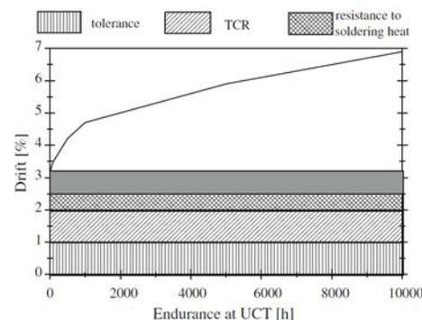
Fig. 1 - Worst case scenario of thick film resistors according to only some of their specifications
