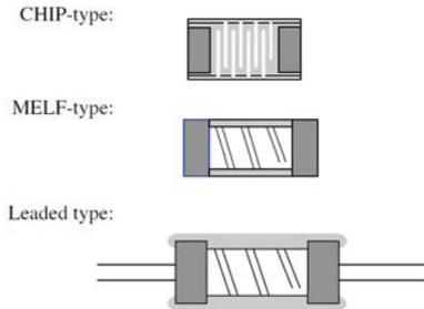
Fig. 4 - Different types of thin film resistors
