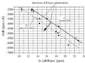
Fig. 12 - Paths of stability - State and rank of all thin film systems and processes are characterised by their position on paths
