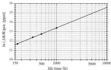
Fig. 9 - time-dependence of  $\ln(\Delta R/R)_{pot}$  for CrSi thin film CHIP resistors size 0603
