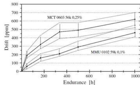
Fig. 5 - Available endurance test data (UCT: 125 °C) in usual graph
