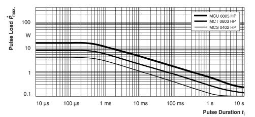
Maximum pulse load, single pulse; applicable if  $\overline{P} \to 0$  and  $n \le 1000$  and  $\hat{U} \le \hat{U}_{max}$ ; for permissible resistance change  $\pm (0.5 \% R + 0.05 \Omega)$
