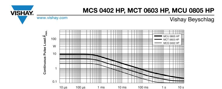
Maximum pulse load, continuous pulses; applicable if  $\overline{P} \leq P(v_{amb})$  and  $\hat{U} \leq \hat{U}_{max}$ ; for permissible resistance change ± (0.5 % R + 0.05  $\Omega$ )
