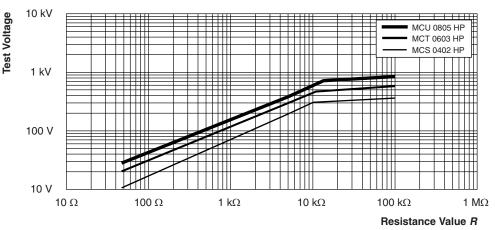
Pulse load rating in accordance with EN 60115-1 clause 4.27; 10  $\mu$ s/700  $\mu$ s; 10 pulses at 1 min intervals; for permissible resistance change ± (0.5 % *R* + 0.05  $\Omega$ )
