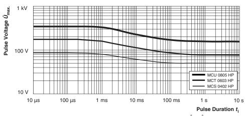
Maximum pulse voltage, single and continuous pulses; applicable if  $\hat{P} \leq \hat{P}_{max}$ ; for permissible resistance change ± (0.5 % R + 0.05  $\Omega$ )
