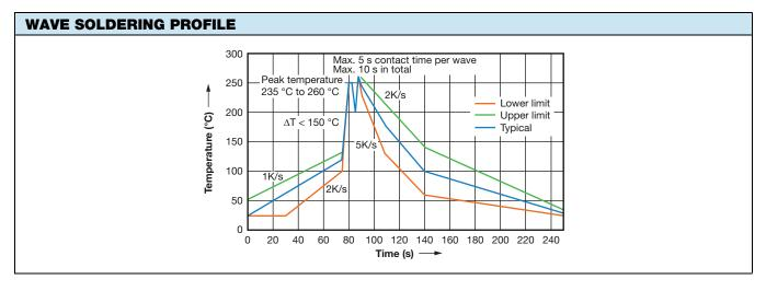
The maximum wave temperature should always be limited to 260 °C, and the total wave immersion time should be limited to 10 s max. In the case of double wave soldering, the total soldering time, including the time between waves, should also be limited to 10 s max.
