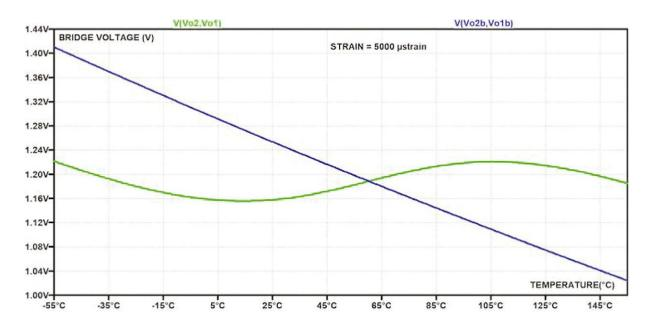
**Bridge Voltage Output vs. Temperature**
