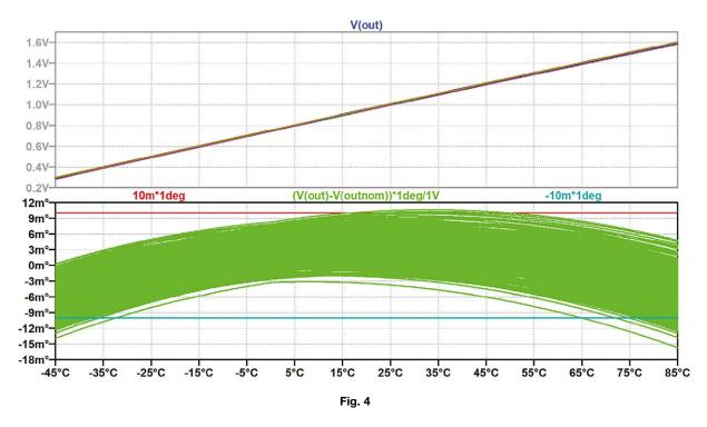
Higher pane: the linear output voltage of the LTC2063 as a function of the temperature.
