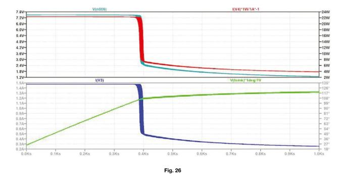
Above this temperature, the current through the load (U2) will be strongly reduced.
