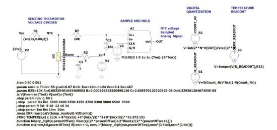
We present the results corresponding to a sample time period of 10 ms and we assume that the ADC bit number is 24. The measured temperature is represented by the voltage source V1, which swings between low and high temperature. The thermistor voltage V(NTC) is then sampled and converted to a digital signal and then transformed into a temperature knowing the Steinhart and Hart coefficients (A, B, C, and D) of the NTCLE317E4103SBA thermistor.
