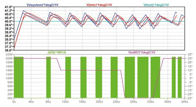
One can visualize the different response of the system depending upon the different element tolerances (Monte Carlo distribution).
