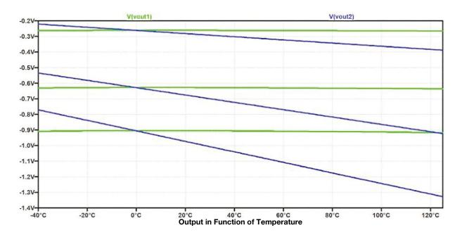
If we introduce the PTS tolerances (TOL $_0$  = 0.6 and TOL $_S$  = 0.01) we can rerun the simulation, and we see the influence of these tolerances on the compensation: for  $V_{IN}$  = 5 V, all the fixed resistors have  $\pm$  1 % tolerance.
