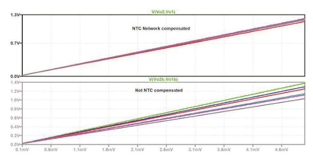
Bridge Output vs. Strain (NTC Compensated Above) and NOT (Under)
