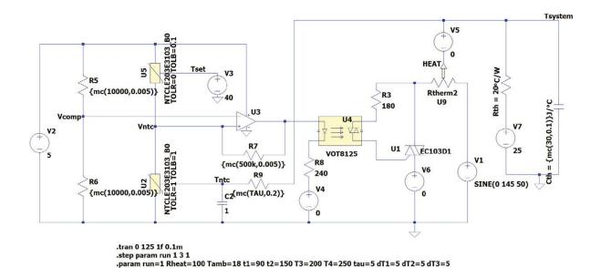
In the thermal circuit of the device / oven we have introduced the ambient external temperature, changing in time from +25 °C to lower temperature. At low temperatures, the duty cycle of the triac on state increases.
