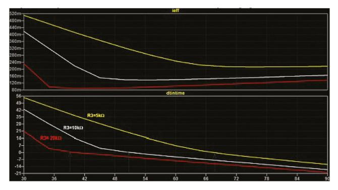
Fig. 8 - Higher Pane: I<sub>RMS</sub> in LED / Lower Pane: Temperature Increase (mK/s) as a Function of Initial LED Temperature (°C)
