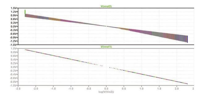
We see that  $V_{OUT1}$  (lower pane) is perfectly stabilized in temperature, and changes linearly as a function of the log of the input voltage. On the contrary,  $V_{OUT2}$  presents a spread in temperature for any fixed  $V_{IN}$ .
