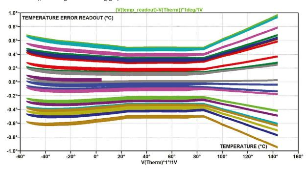
This accurately reproduces the two-point sensor's precision ( $\pm$  0.5 °C between +25 °C and +85 °C, and then increasing up to  $\pm$  1 °C around +140 °C).
