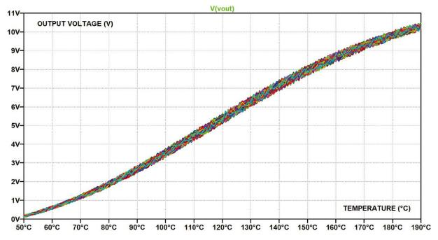
In the SPICE error log file, the temperature span corresponding to a real +185 °C temperature can be evaluated around +182 °C to +188 °C. The user can thus evaluate if the decreased tolerance (price increase) is worth the value of the improved accuracy.
