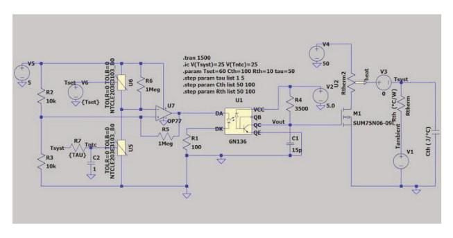
Thermostat Based on 6N136 and Thermistor
