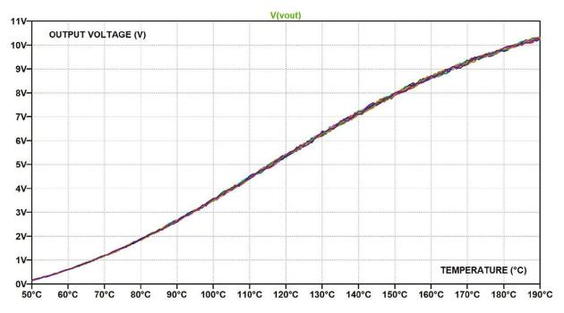
It is then possible with some SPICE directives to determine the accuracy of the  $V_{OUT}$  measurement: at +185 °C,  $V_{OUT}$  is equal to 10.06 V nominally. Introducing tolerances for the circuit elements, we can then compute at which temperature span the  $V_{OUT}$  voltage will cross 10.06 V. The SPICE error log file allows for visualization of this span, which will swing between +183 °C and +187 °C, thus +185 °C  $\pm$  2 °C, values near the specification.
