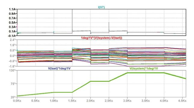
The analysis can be done as a worst-case analysis or Monte Carlo random, or here a combination of both distributions. It is possible to visualize temperatures in LTspice XVII by multiplying the corresponding voltages by a factor of (1° / 1 V). The scale is then transformed magically into °C.
