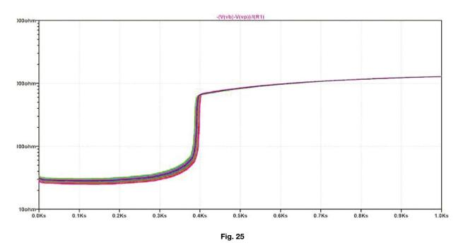
Fig. 25 represents the PTC resistance variation in time showing the strong resistance increase at a defined temperature (here between +115 °C and +120 °C) (Fig. 26).
