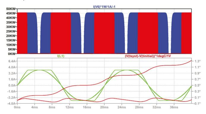
At high temperature, the duty period is reduced: the IGBT switching is derated, which induces less heat into the heatsink and the temperature stabilizes. More information about the simulation can be obtained at <a href="mailto:edesign.ntc@vishay.com">edesign.ntc@vishay.com</a>
