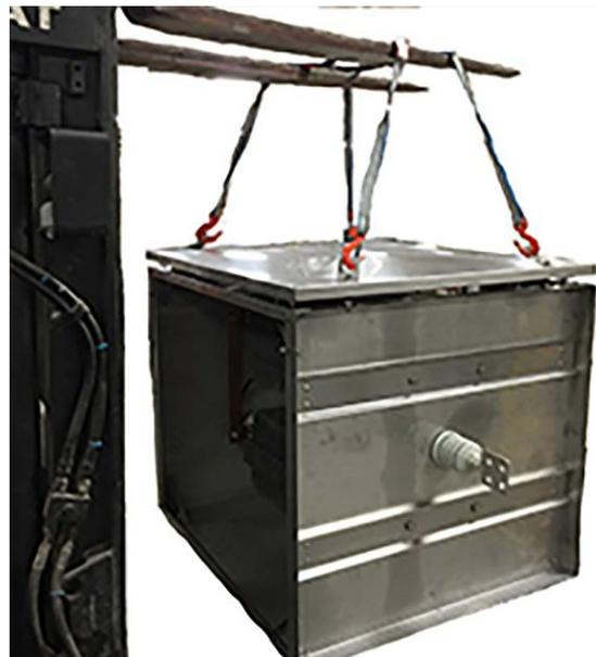
Example of lifting from top via fork lift
