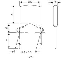
Component outline for lead spacing 2.5 mm ± 0.8 mm lead spacing 5.0 mm  $\pm$  0.8 mm (flat bent leads)
