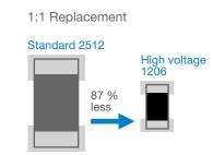
**Voltage Coefficient** — The voltage coefficient of resistance (VCR) indicates the resistor's permissible change of resistance, depending on the operating voltage. Hence, using high voltage resistors at the allowed elevated voltage levels may cause a significant resistance change. Thus, high precision applications will benefit from thin film resistors, which feature an especially low VCR of  $\leq$  2 ppm/V.
