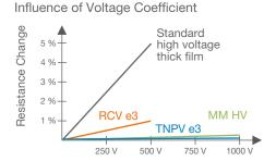
TNPV e3 — TNPV e3 high voltage thin film flat chip resistors combine high voltage ratings with thin film technology advantages: tight tolerance, low temperature coefficient, and excellent long term stability.
