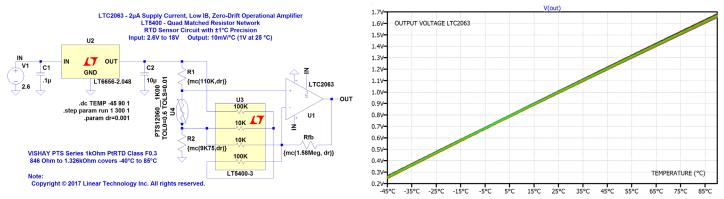
Fig. 1 - LTspice Simulation of Opamp LTC2063 Linear Output With PTS Sensing
