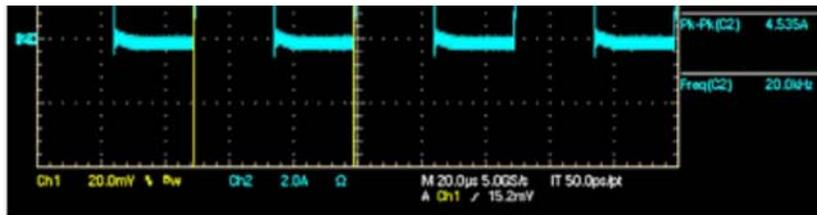
Fig.1. Step Response of SiP12107. VIN = 5 V, VOUT = 1.2, Fsw = 2 MHz; Load step at 20 kHz = 0 to 3 A; L = 330 nH, CIN = 22 µF, COUT = 22 µF; Yellow = VOUT, Blue = current.
