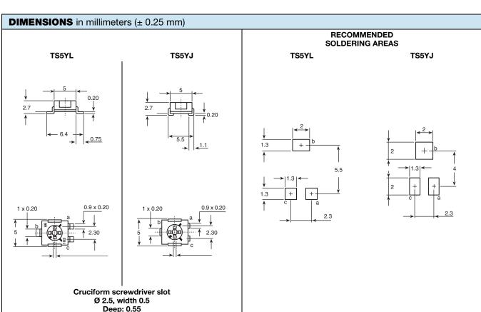
The TS5 trimming potentiometer has been designed for surface mount applications and offers volumetric efficiency (5 mm x 5 mm x 2.7 mm) with high performance and stability.
