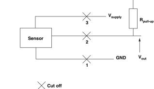
$V_{\text{pull-up}} \, \text{can be independent to} \, V_{\text{supply}}$
