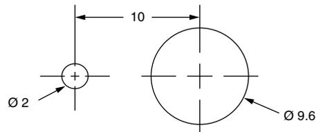
Fig. 1 - Panel drilling (mm)
