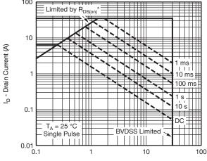
$\rm V_{DS}$  - Drain-to-Source Voltage (V)  $^*$  V  $_{GS}$  > minimum V  $_{GS}$  at which  $\rm R_{DS(on)}$  is specified Safe Operating Area, Junction-to-Ambient
