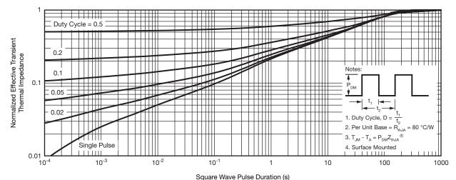
Normalized Thermal Transient Impedance, Junction-to-Ambient
