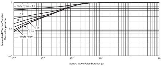
Normalized Thermal Transient Impedance, Junction-to-Case
