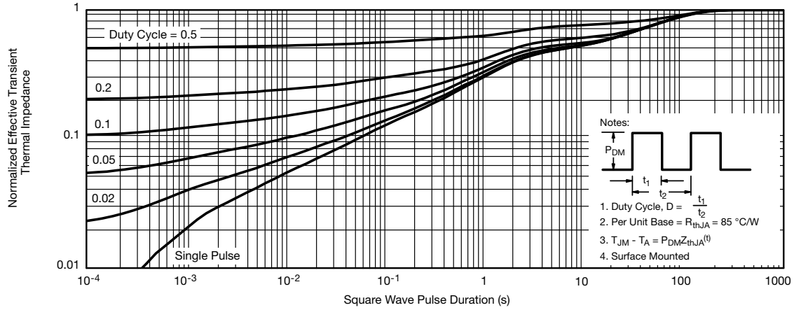
Normalized Thermal Transient Impedance, Junction-to-Ambient
