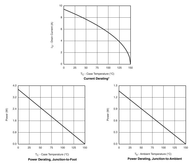
\* The power dissipation P<sub>D</sub> is based on T<sub>J(max)</sub> = 150 °C, using junction-to-case thermal resistance, and is more useful in settling the upper dissipation limit for cases where additional heatsinking is used. It is used to determine the current rating, when this rating falls below the package limit.
