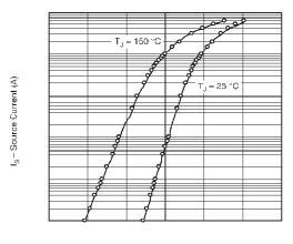
V... = Source-to-Drain Voltage (V)
