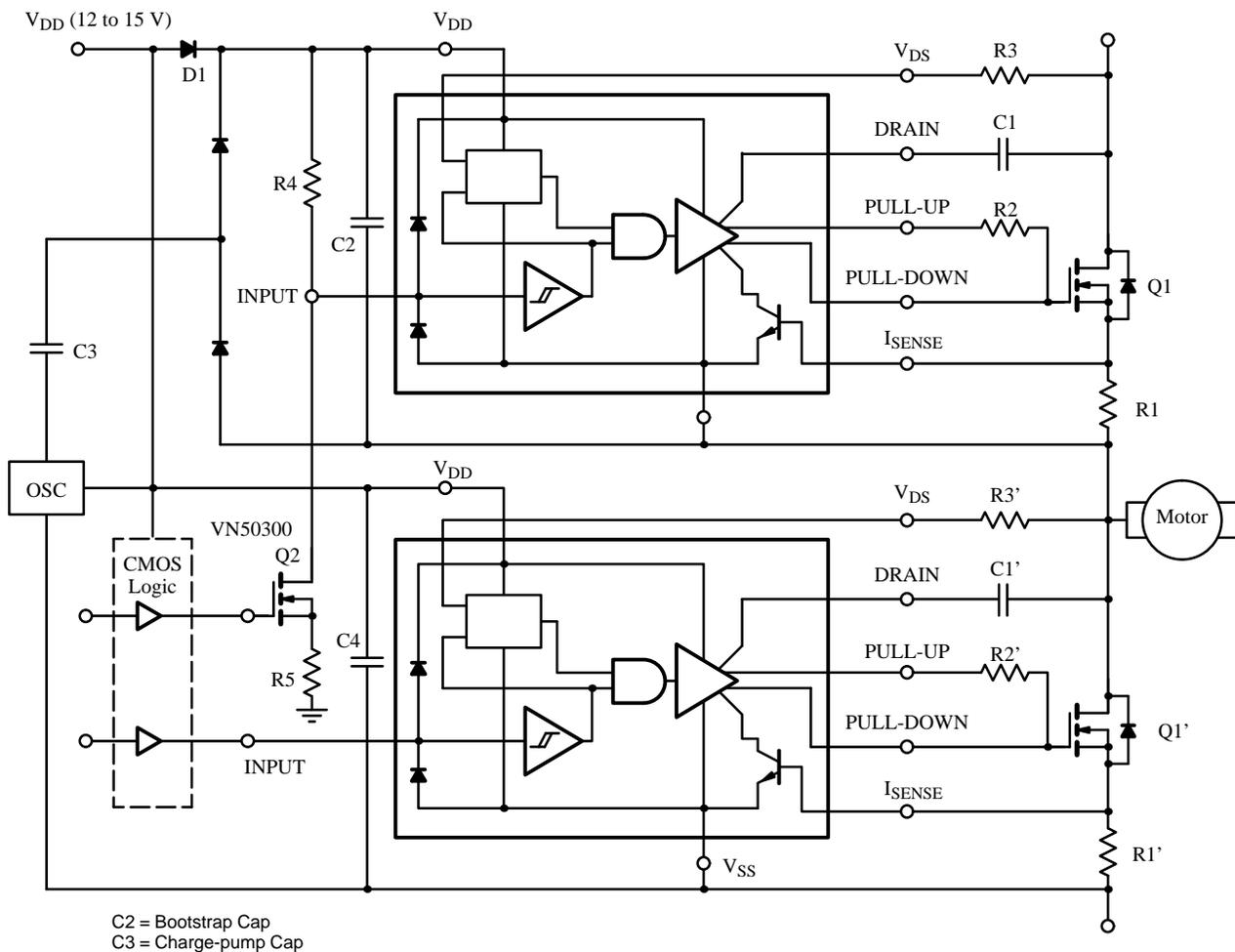
Figure 4. Si9910DY Adaptive MOSFET Gate Driver
