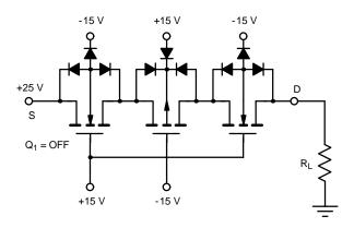
FIGURE 10. The 3-FETs-in-Series Channel Offers Inherent Fault Protection
