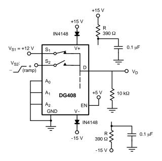
FIGURE 6. Overvoltage Test Circuit
