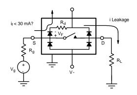
**FIGURE 2.** Fault Current Flows When  $V_q > V_+$
