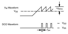
Figure 7. Load Detection in Overcharge Mode
