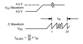
Figure 4. DL2 Time (Over-Charge)
