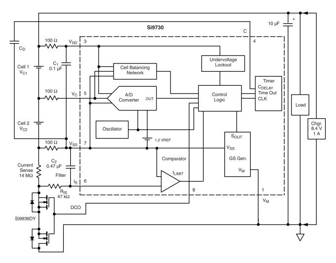
Figure 8. Typical 2 -Cell Circuit
