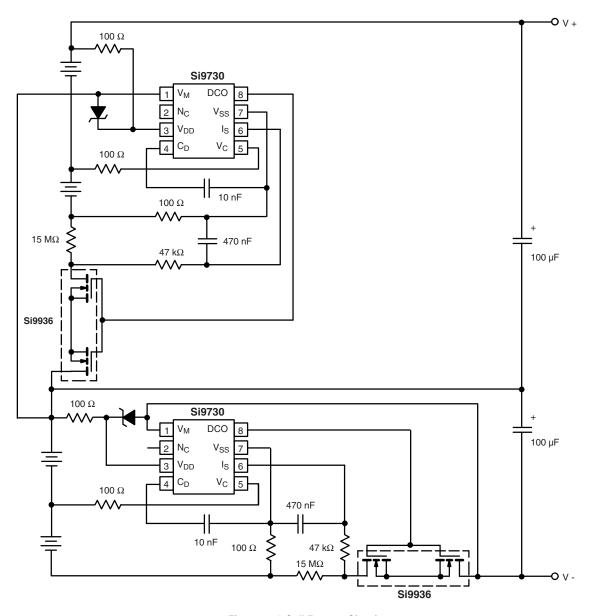
Figure 9. 4-Cell Battery Circuit
