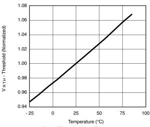
Reset Threshold vs. Temperature
