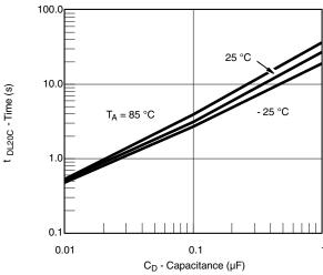
DL2 Period (Over Discharge) vs. Capacitance
