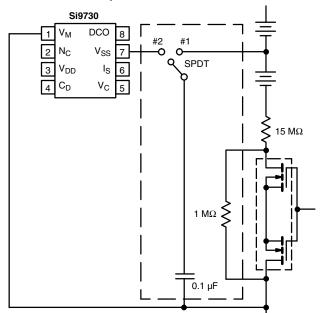
Figure 10. Factory Startup Circuit
