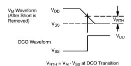
Figure 3. Reset Threshold
