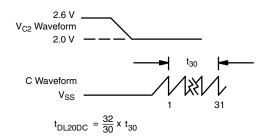
Figure 5. DL2 Time (Over-Discharge)
