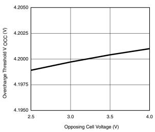
Overcharge Threshold vs. Opposing Cell Voltage
