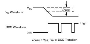
Figure 6. Power-Down Charger Detect Threshold
