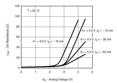
r<sub>ON</sub> vs. V<sub>B</sub> Single Supply Voltage
