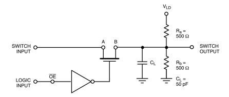
Input driven by 50  $\Omega$  source terminated in 50  $\Omega$  C<sub>L</sub> includes load and stray capacitance Input PRR = 1.0 MHz,  $t_W$  = 50 ns
