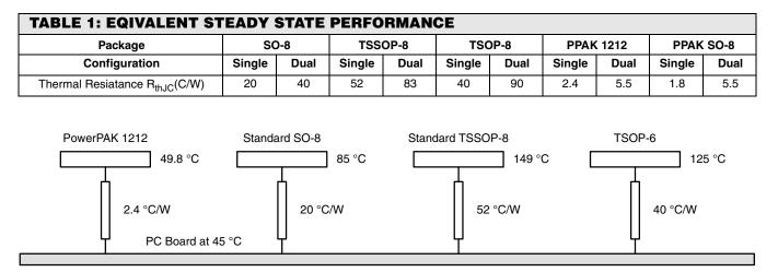
Figure 4. Temperature of Devices on a PC Board
