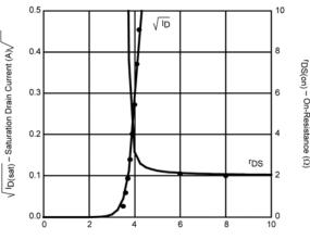
V<sub>GS</sub> – Gate-to-Source Voltage (V)
