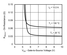
On-Resistance vs. Gate-to-Source Voltage
