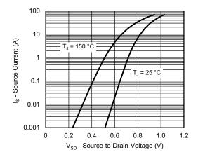
Source-Drain Diode Forward Voltage
