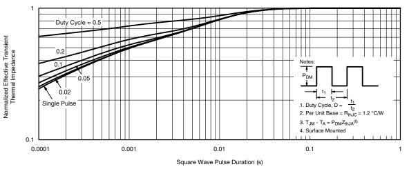
Normalized Thermal Transient Impedance, Junction-to-Case
