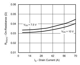
On-Resistance vs. Drain Current and Gate Voltage
