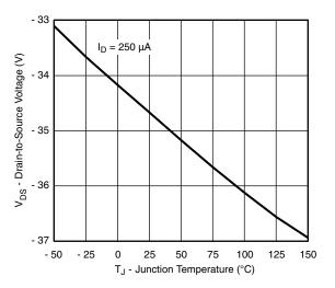
Drain Source Breakdown vs. Junction Temperature
