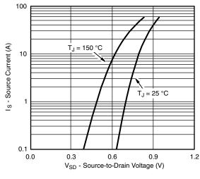
Source-Drain Diode Forward Voltage
